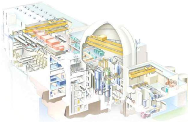
200MW CFBC Power Plant Cutaway
