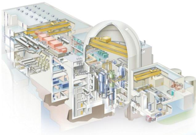
200MW CFBC Power Plant Cutaway
